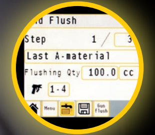
Function "Last A material" prevents sticking of the valve seat and thus avoids a standstill.
